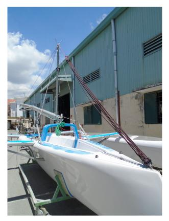
Check to see that all rigging wires are clear and have not snagged anywhere. Raising wires should initially be slightly loose and tighten slightly on the way up.
