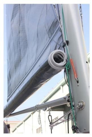
Once you have connected the boom onto mast. Attach the adjustable boom topper onto the rotating SS bracket on the out board end of boom.
